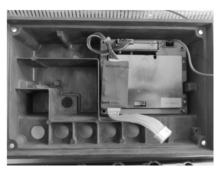
The original cable is attached to the GPS Receiver side. The cable that comes with the kit is attached to the GPS mainboard side.
