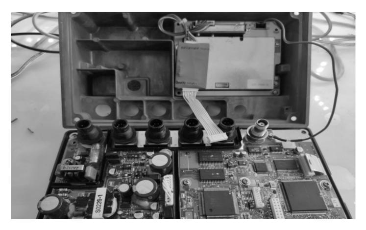
Make sure the connectors are fully inserted into their sockets.
